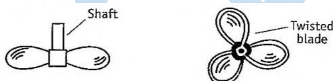
(a) Side view (b) Top view (Propeller type of mixing devices. A three bladed design.)
